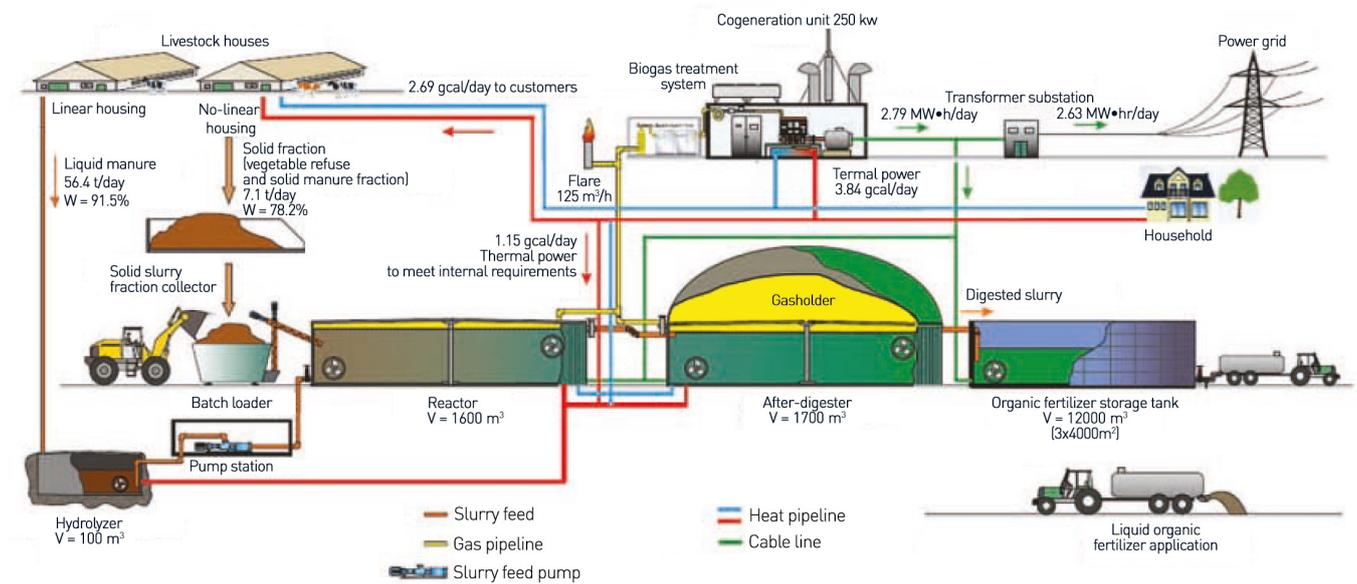
Fig.1. Biogas plant flow chart
