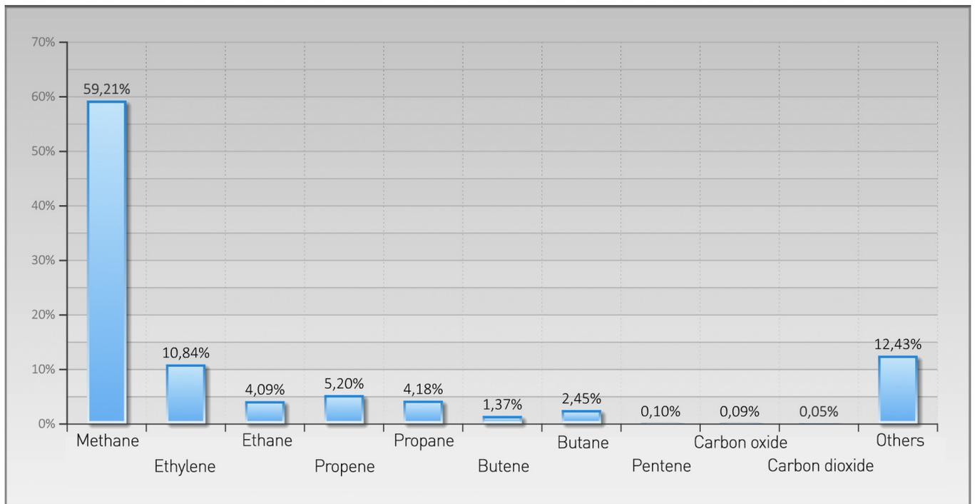
Fig.5. Pyrolysis gas content.
