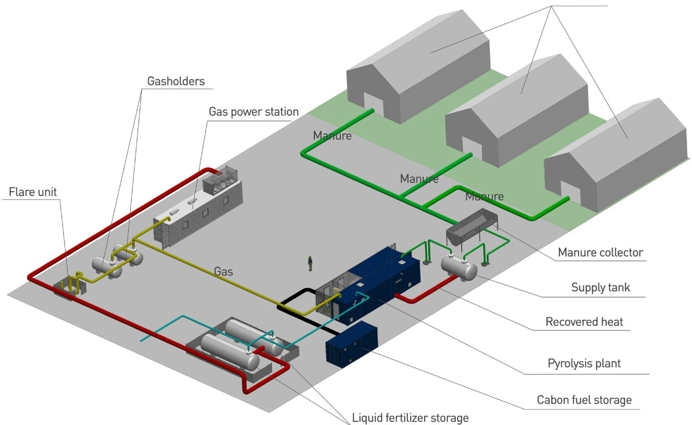
Fig.3. Pyrolysis plant layout diagram.
